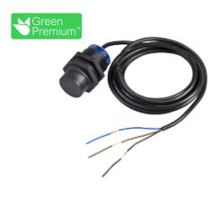
Inductive proximity sensors XS, inductive sensor XS4 M30, L53mm, PBT, Sn15mm, 24...48 VDC, cable 2 m
