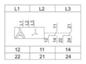
L1,L2,L3 : Supply to be monitored 11-14,12 : 1st C/O contact of output relay 21-24,22 : 2nd C/O contact of output relay **Technical Description**
