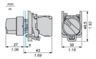
e: clamping thickness: 1 to 6 mm / 0.04 to 0.24 in.
