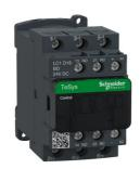
IEC contactor, TeSys Deca, nonreversing, 18A, 10HP at 480VAC, up to 100kA SCCR, 3 phase, 3 NO, 24VDC coil, open
