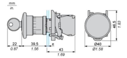
e : clamping thickness: 1 to 6 mm / 0.04 to 0.24 in.
