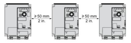
Only Possible at Ambient Temperature Less or Equal to 50 °C (122 °F)
