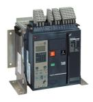
Circuit breaker frame, MasterPact NT10H1, 1000A, 42kA/440VAC 50/60Hz (Icu), 3 poles, drawout, without control unit
